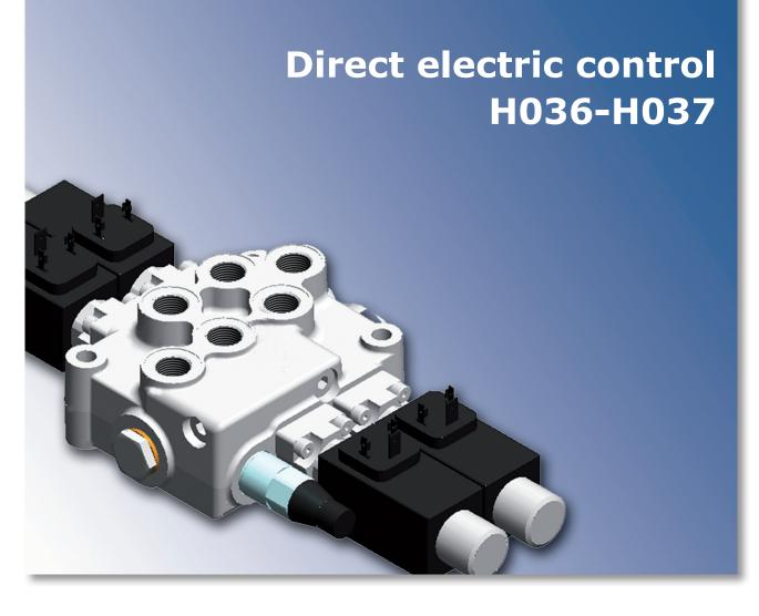
The ON-OFF electric control for HC-M45 control valves is equipped with two push-push magnets to apply a direct thrust to both ends of the spool.
